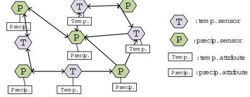
**Figure 3: Illustration of Weather Sensor Information Network**
